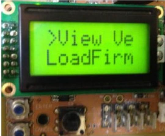
**Figure 5: Load Firmware (Selected to do Firmware Updates from USB)**
